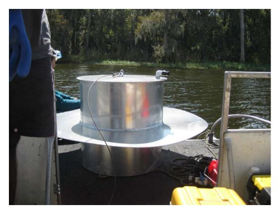
Figure 2-3. Typical Seepage Meter Used in Lake Jesup.
