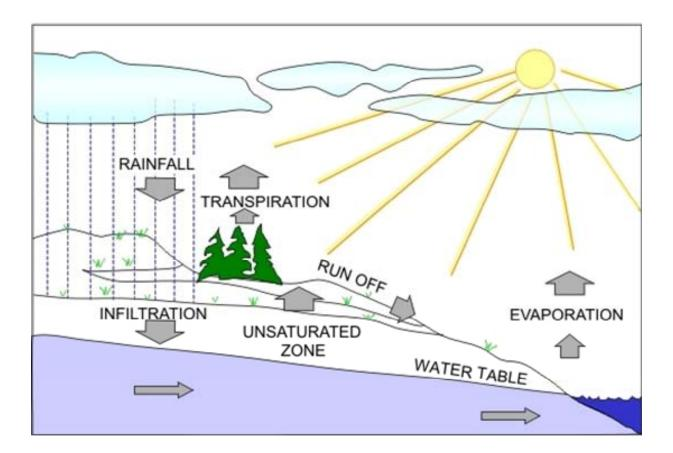
Figure 2-1. Hydrologic Cycle Illustrating Groundwater Seepage to Surface Waters.
