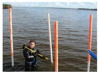
Cylinder inserted into sediments using sledge hammer
